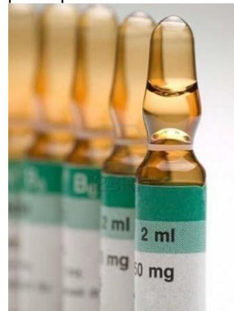
Ampoules used to store biohazardous material in liquid nitrogen have exploded causing eye injuries. The use of polypropylene tubes eliminates this hazard. These tubes are available dust-free and pre-sterilized and are fitted with polyethylene caps and with silicone washers. Heat sealable polypropylene tubes are also available.
