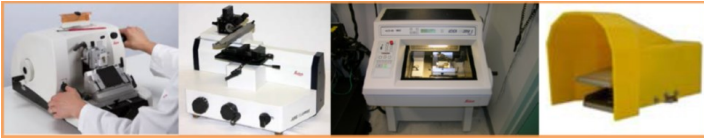
(l to r) Rotary, Sliding and Freezing (Cryostat) microtome and foot treadle guard
