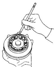
Figure 2. Checking the rotor web area.
