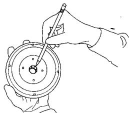
Figure 1. Checking the rotor hub.
