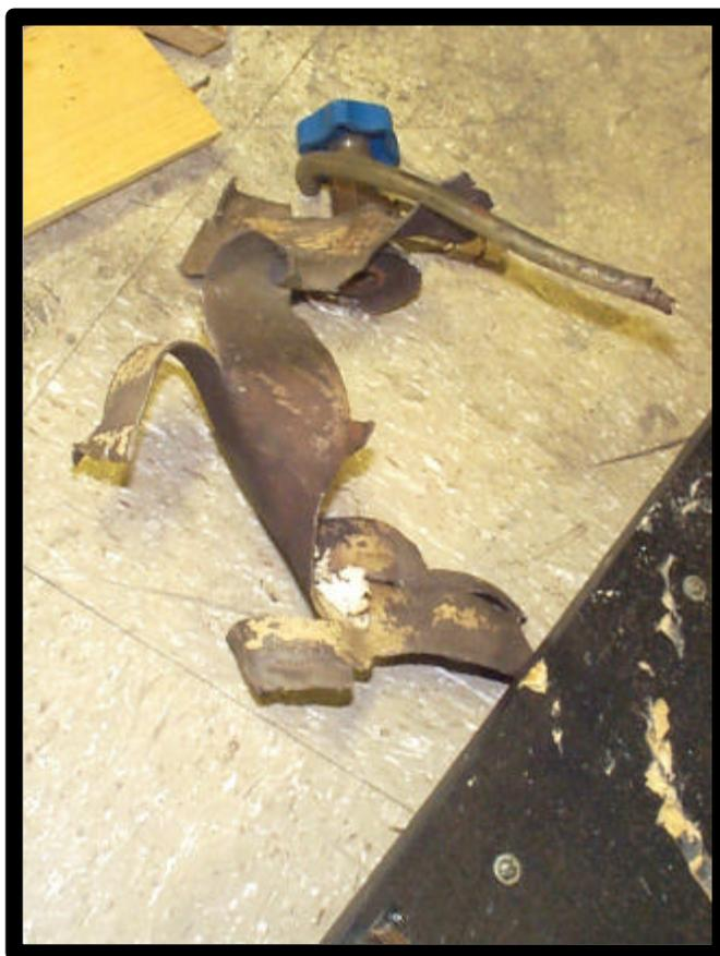
Ruptured Gas Cylinder
