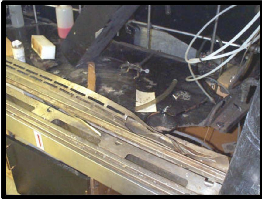
**Gas cylinder was propelled through hood airfoil**
